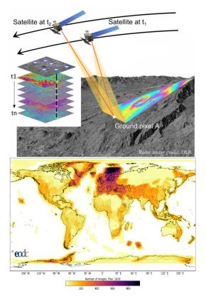
Fig. 1. InSar Presentation: **top**: the satellites imaging the same place at different times, hence allowing to build a stack of radar interferograms which are differentiation of the phase of radar images. **bottom**. Density of image acquisition. Revisiting time goes up to 2 days in Europe.
